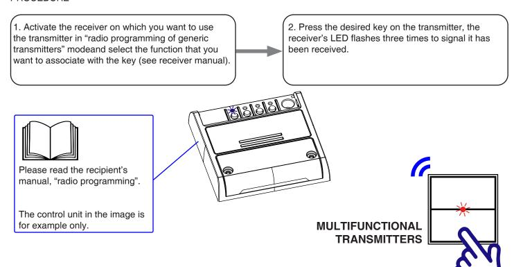
**ACTION:** Send a command from the transmitter **RECEIVER LED:** Flashes 3 times
