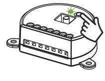
**ACTION:** Short pressure RADIO button **LED:** Flash
