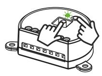
ACTION: Long press of buttons RADIO e Wi Fi LED: Turns on green
