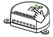
ACTION: Short pressure Wi Fi button LED: Turns off
