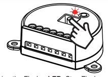
ACTION: Short pressure of button Wi Fi during the Flash LED: Stop Flashes
