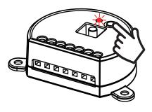
**ACTION:** Short press of button RADIO **LED:** Flashing quickly and turns off
