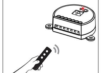
**ACTION:** Make a transmission with the transmitter **LED:** Flashing quickly and turns off
