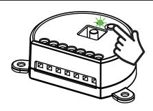
ACTION: Short pressure RADIO button LED: Turns off
