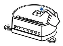
ACTION: Short pressure RADIO button LED: Flash
