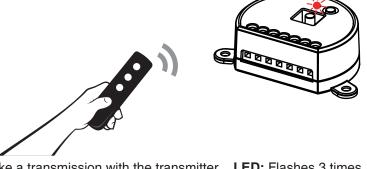
**ACTION:** Make a transmission with the transmitter LED: Flashes 3 times
