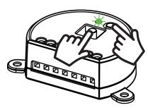
ACTION: Long press of buttons RADIO e Wi Fi LED: Turns on green/blu
