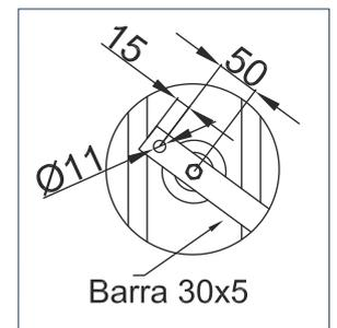
TERMINALI BASSA TENSIONE (BT) - TERMINALS AT LOW VOLTAGE (LV)
