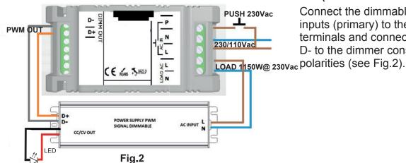
Connect the dimmable electronic driver inputs (primary) to the dimmer LOAD terminals and connect the inputs D+ and D- to the dimmer considering the
