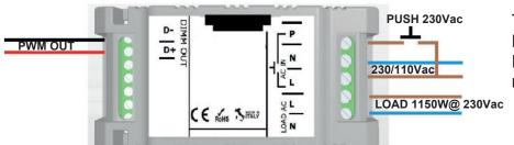
The device can be controlled with a PUSH-button.
