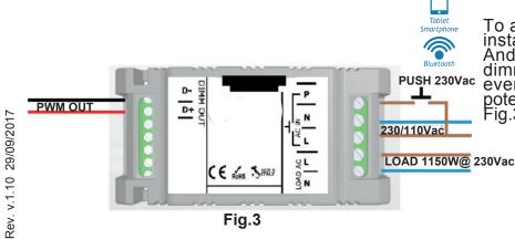
To activate such modality, it is required to install the LEF Lighting App on the Android or iOS device selected for dimmer control and to disconnect eventual 0-10V (1-10V) signals or potentiometer connected to dimmer (see Fig.3).
